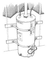
Water heaters can move or tip over if not securely anchored to the wall or floor. For a small investment of time and money, you can avoid spilling gallons of precious water that could be useful in an emergency.
